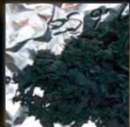
The finished product. Carbon nanotubes don't look like tubes at all to the naked eye. They are so tiny that they resemble flecks of black powder.
